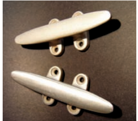
Aluminum deck cleats clean up nicely with a little judicious sanding, brushing and buffing, left and right. Stainless-steel gudgeons, below, also respond to TLC and will enhance the boat's appearance when re-installed.
