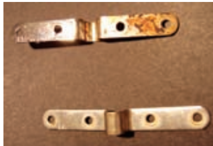
Aluminum deck cleats clean up nicely with a little judicious sanding, brushing and buffing, left and right. Stainless-steel gudgeons, below, also respond to TLC and will enhance the boat's appearance when re-installed.
